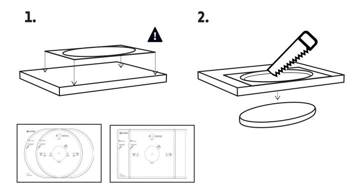
Use the template, in the package, to help you with the right installation dimensions when cutting into your table top. Please note that the installation requires a water trap and a separate drainpipe depending on the site.
