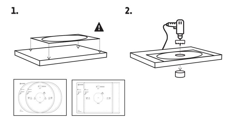
Use the template, in the package, to help you with the right installation dimensions when cutting into your table top. Please note that the installation requires a water trap and a separate drainpipe depending on the site.
