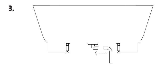
The installation requires a separate drainpipe depending on the site.
